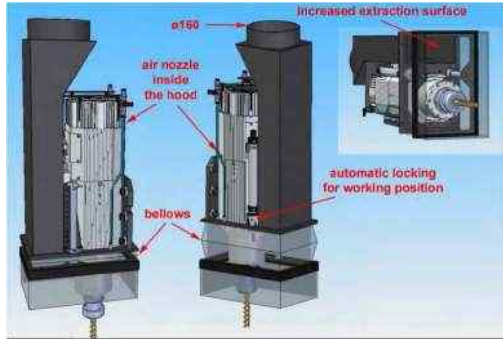
CN CONTROLLED DUST EXTRACTOR BELLOW
